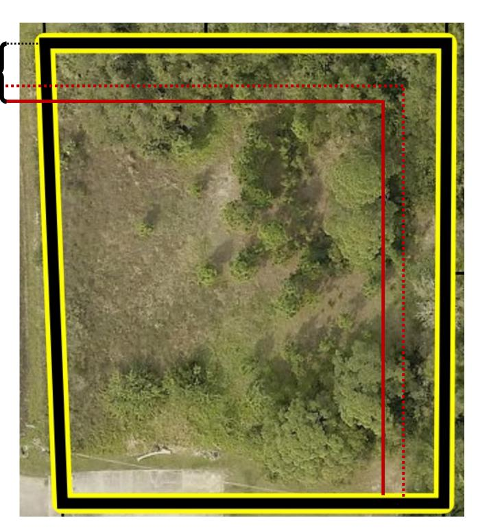
In addition to veg. buffer and use buffer: 8' (from finished floor elevation) OR 12' (from filled grade) <u>OPAQUE</u> FENCE (applicant's choice of PVC or wood) installed at 25' use buffer along N & E
