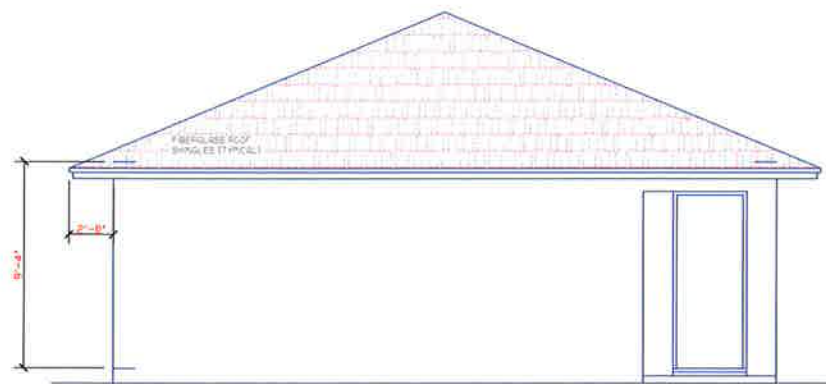
GUEST HOUSE LEFT SIDE ELEVATION SCALE: 1/4" = 1'-0"
