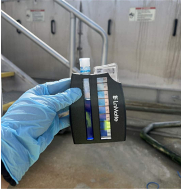
Figure 3-3 Photo 1 - Wastewater Sulfides and pH
