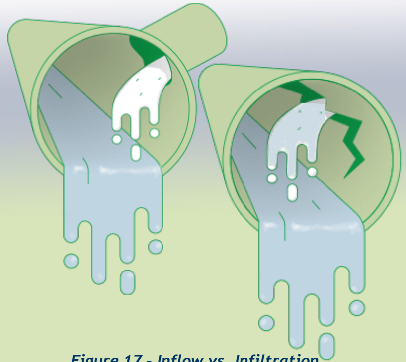
Figure 17 - Inflow vs. Infiltration
