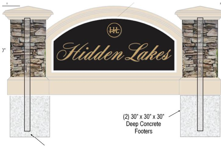
Note: Undisturbed Sandy Soil w/ Min. Lateral Soil Bearing Pressure = 150 psf/ ft of depth. If soil conditions differ notify Engineer to re-size footers.
