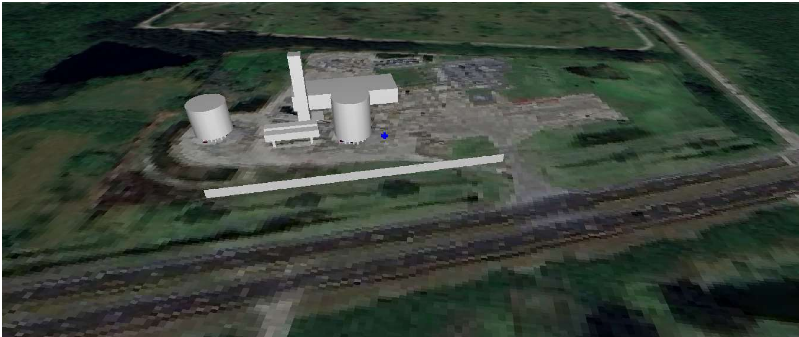
FIGURE 1. Acoustical model depiction of a 14 foot barrier along current fenceline. Barrier is approximately 400 feet long.
