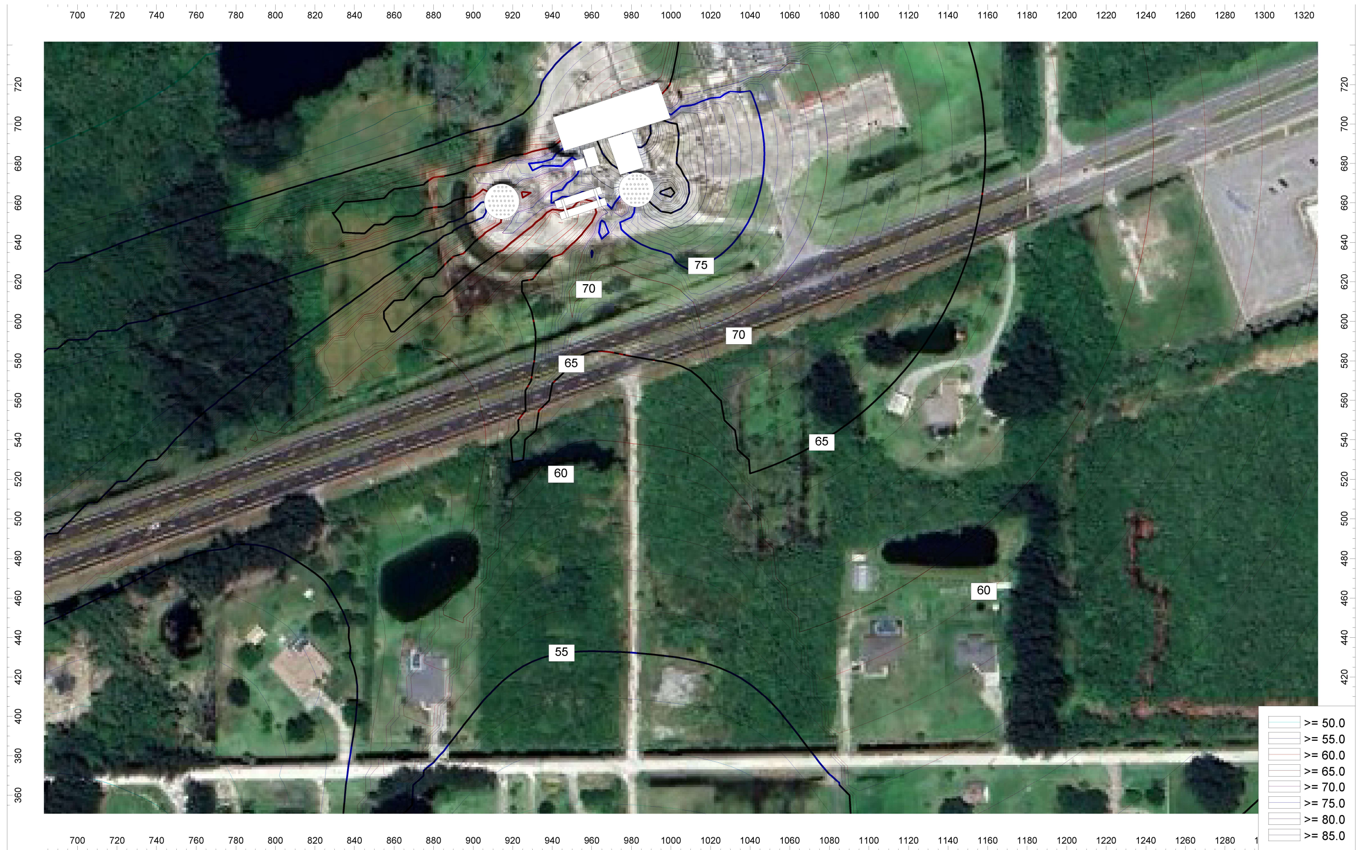
Figure 2. Modeled Noise Propagation from Two noise sources: LSS and Pump Truck.
