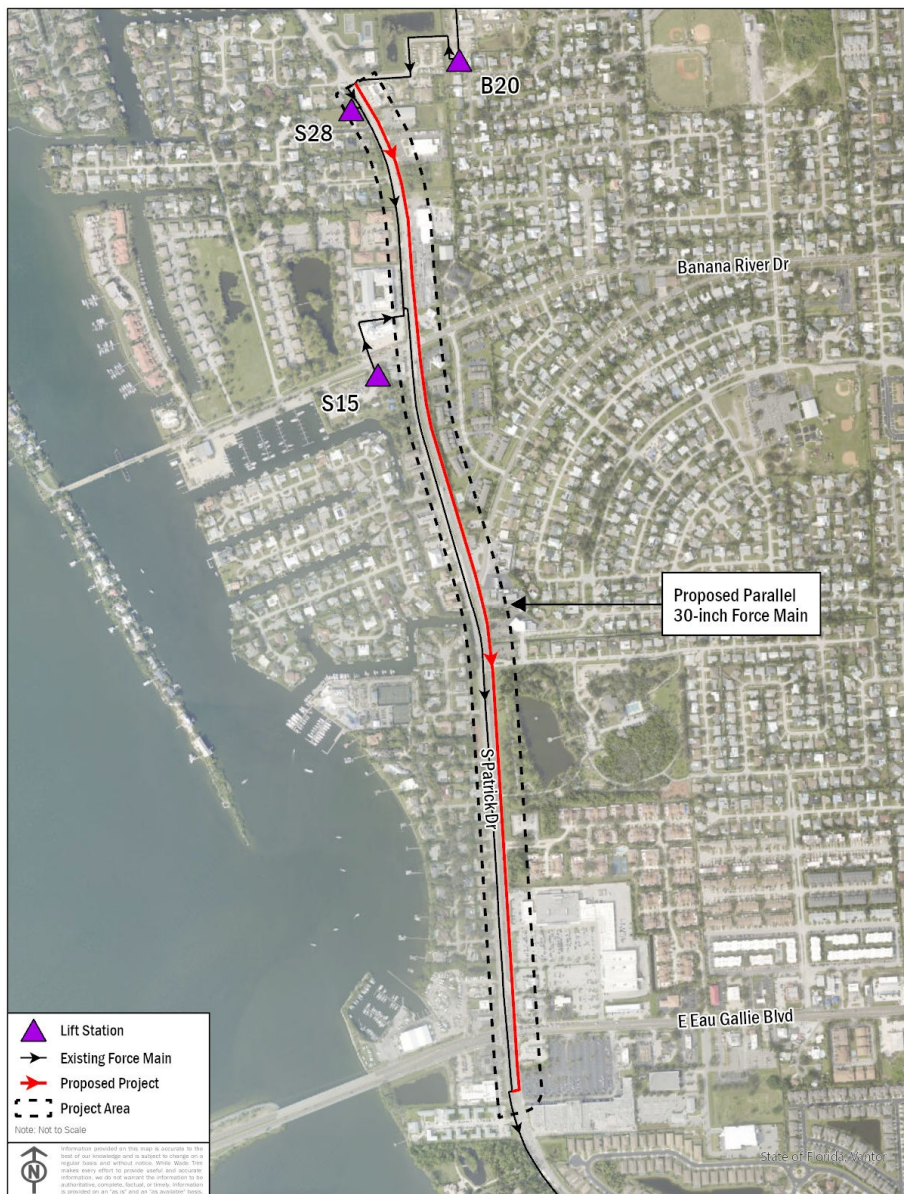
Figure 5-1. Proposed Wastewater Improvements
