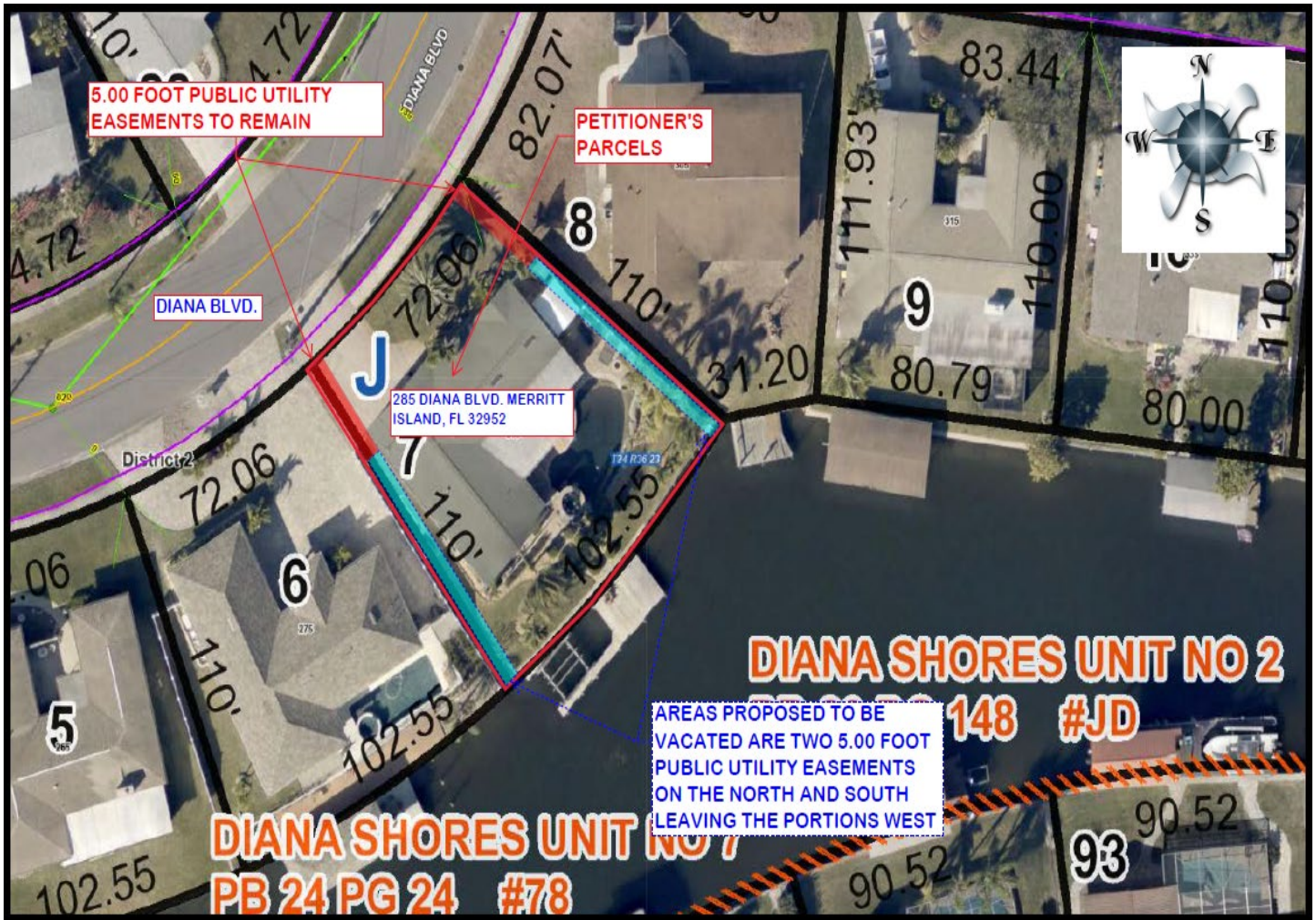
Figure 2: Aerial Map for easements to be vacated at Lot 7, Block "J", Diana Shores Unit No. 2, Merritt Island.
