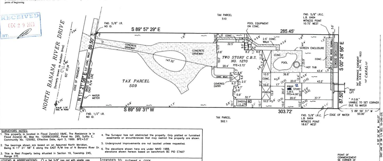
LEGEND & ABBREVIATIONS: O = Set 5/8" iron rod with plastic cap △ = Set noil with metal disc □ = Set concrete monument with disc ----- = Center Line – := 4' C.L.F. XXX = Existing Elevations -=6' W.E.
