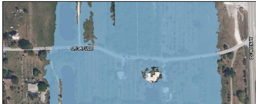
Figure 8.2: 10-Year, 24-hr Floodplain along W. Crisafulli Rd.
