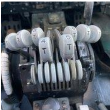
Throttle quadrant (eight jet engines) from B-52 cockpit.
