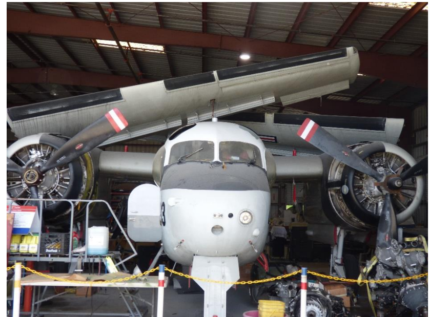
Grumman S2F Tracker, awaiting restoration to flight status (new Wright R1820 engine lower right)
