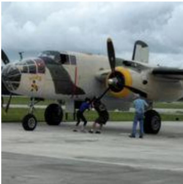
Airworthy B-25 Mitchell bomber "Killer Bee". Owner, master restorer and pilot Tom Reilly overseeing propellor pull-through.
